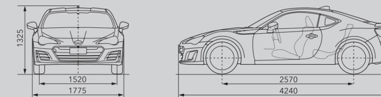
Dimensions are measured in accordance with standard measurement of SUBARU CORPORATION.
